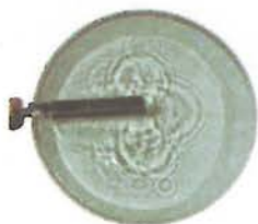
Fig. 10.4: (c) A prong of vibrating tuning fork touching the surface of water
