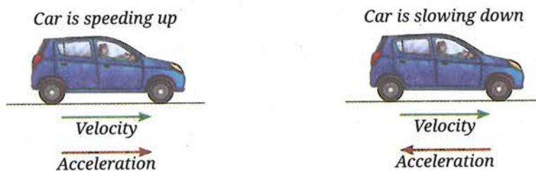
Fig. 4.8: Direction of average acceleration when magnitude of velocity is (a) increasing, and (b) decreasing
